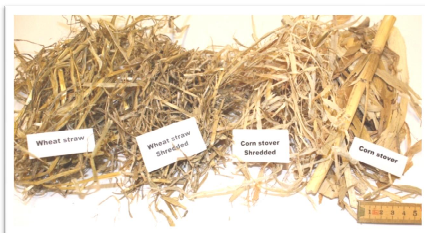
Figure 2: Wheat straw and corn stover before and after mechanical pretreatment (shredding)
